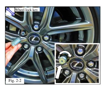
(b) Take the key supplied in the wheel lock set and place it on top of the wheel lock. Turn the lock until the patterns engage (Fig. 2-2).
