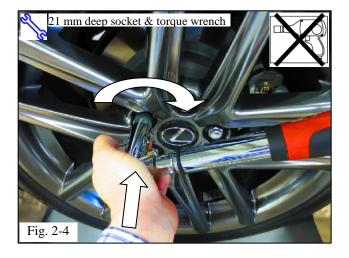
(d) Apply pressure on the key and use a torque wrench to tighten the wheel locks to 103 N·m (76 ft·lbf) (Fig. 2-4).
