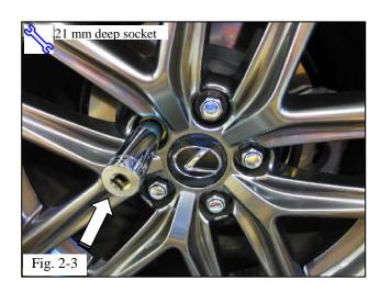
(c) Place the 21mm deep socket on top of the key (Fig 2-3).
